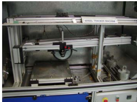
Figure 4: Laboratory wheel tracking for deformation characteristics
