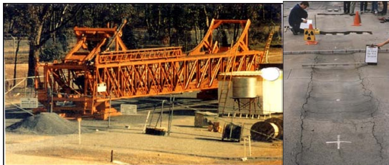
Figure 6: ARRB Transport Research Accelerated Loading Facility
