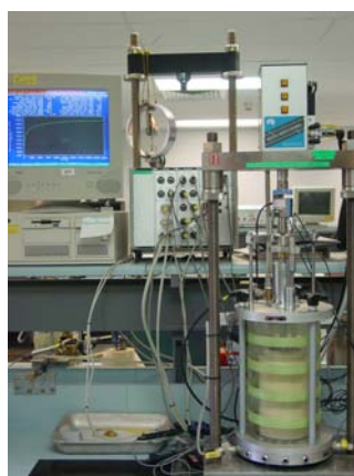
Figure 2: Laboratory dynamic testing of pavement materials
