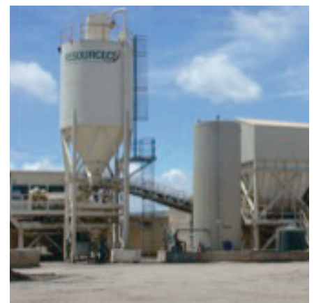
Figure 2. Pug mill with cement and heated emulsion silos for manufacture of Bitumix
