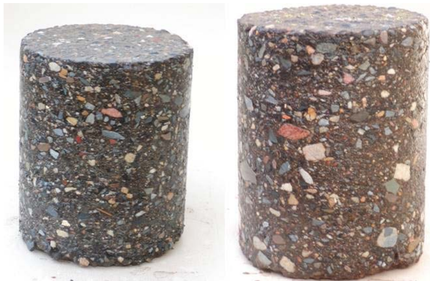
Figure 12 Cores – (1) 175 mm of 14 mm Bitumix and (2) 50mm of 14mm Bitumix and 125 mm of 20 mm Bitumix
